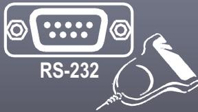
Scanner (powered by the scale)
