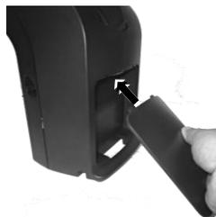
6. Determine that the protective cover is well wedged to the wedge portions of the rear cover of the dock station. Then, gather the I/O cables together for cable arrangement
