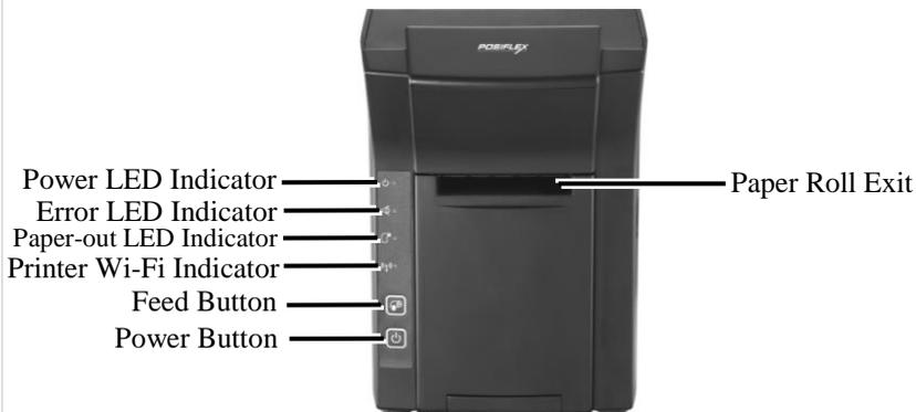
※ **Error LED Indicator, Paper-out LED Indicator, Printer Wi-Fi Indicator, Feed Button, and Paper Roll Exit are provided for DS-210/220/310/320 only.**
