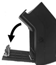
3. Drop the 80mm-wide thermal paper roll inside the paper roll compartment of the printer, as shown in the right figure.
