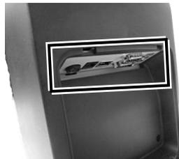
5. Make the protective cover join to the wedge portions of the rear cover of the dock station.
