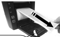
5. To avoid the printing problem occurring, push the central portion of the paper roll cover to close, and make the tail of the paper roll come out of the track between the paper roll cover and the front cover.
