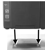
3. Push hard the dock station backward along the 2 tracks of the bracket on the table to firmly secure the dock station.
