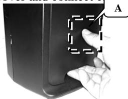
2. Pull the protective cover in the direction indicated by the arrow in the right figure.
