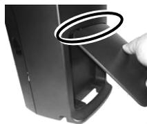
7. Cover the I/O ports of the dock station with the protective cover.
