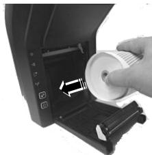
4. Drag the paper roll to the portion where the paper cutter is installed.
