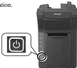
2. The power LED indicator stays bright and solid blue when the dock station is powered ON.
