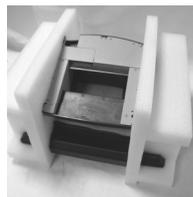
After take the PE foam out from the carton, please remove the PE foam with extra care and make sure place the monitor and stand on a soft clean flat surface such as table and as show in the picture at the right side.
