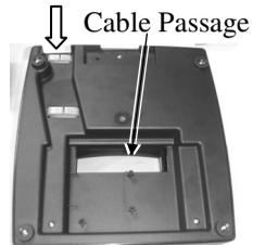
Hook the main unit back onto base stand assembly by matching the matching pegs to round part of matching holes and slide them down to slot part till the rear lock/release button clicks.
