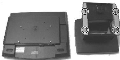
Please find the four holes in the top of stand. Take the stand and align these four matching holes to the four matching pegs which are in the back on monitor.
