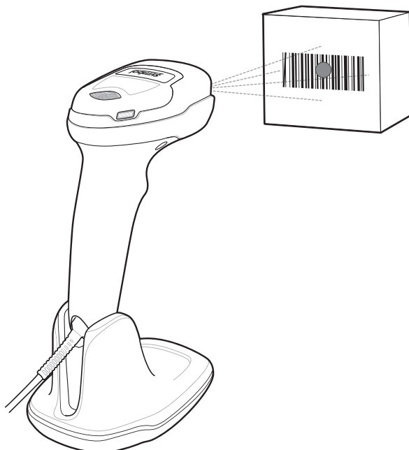
Figure 2-8 Scanning with the DS4308P
